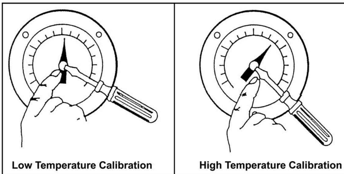
3. If it does not match, remove the dial thermometer lens with a small screwdriver.
