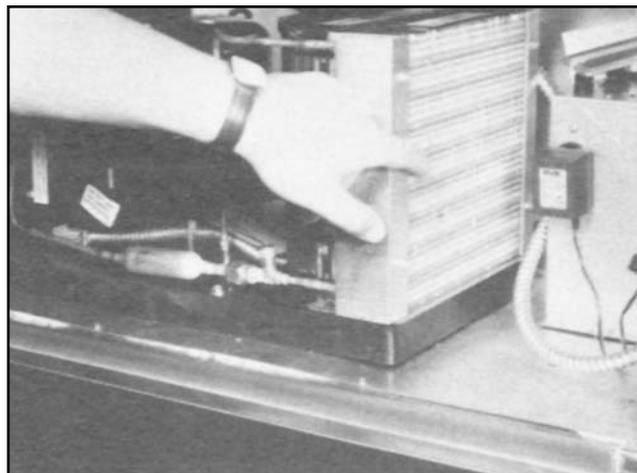
**WARNING: Failure to keep condenser clean may cause premature failure of motor-compressor which will NOT be covered by warranty.**
